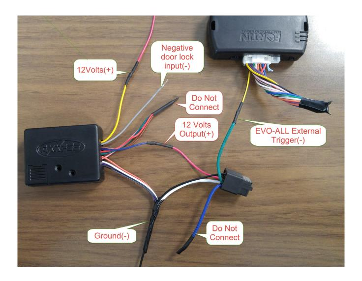
Note: The Gray (Pin 10) wire from the Metra Axxess Trigger will need to be connected to the door lock motor wire that will pulse ground (negative) every time you push LOCK on the OEM remotes.
